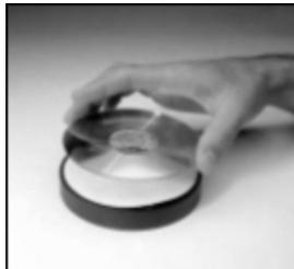
Holding CD disc by the edges, place over center post of plunger. **DATA SIDE UP!**
